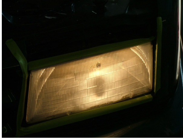
Photo 1. Deteriorated PC head light where the light performance audit shows only 3,000 Candela on low beam and 7,000 Candela on high beam (Candela definition; unit of luminous intensity)
