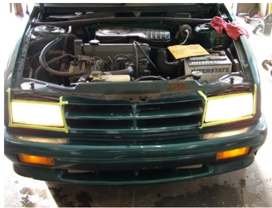
Photo 3. PC Headlights that have been refinished with an OEM style UV-A hard coat
