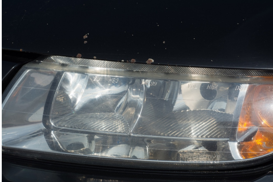
Photo 4. 36 months of service in the North Eastern part of the US shows limited degradation to the OEM Style Refinishing UVA Cured Hard Coat.
